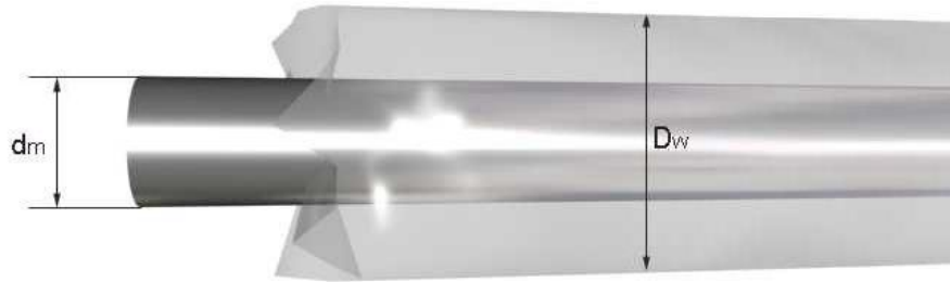
Fig. 2. Glass-coated magnetic microwires, where d_m = 2 r_m ( r_m is the radius of metallic core of the microwire) and D_w = 2 R_w ( R_w the total radius of the CGCMNW).
