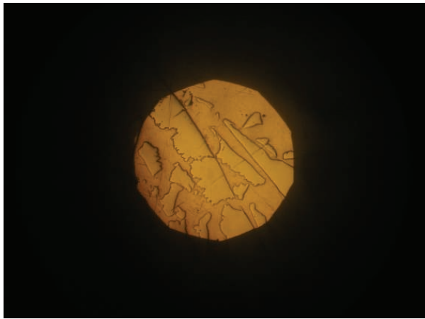
Fig. 3. Metallographic sample of the transverse cross-section of Bi microwire with Fe inclusions.
