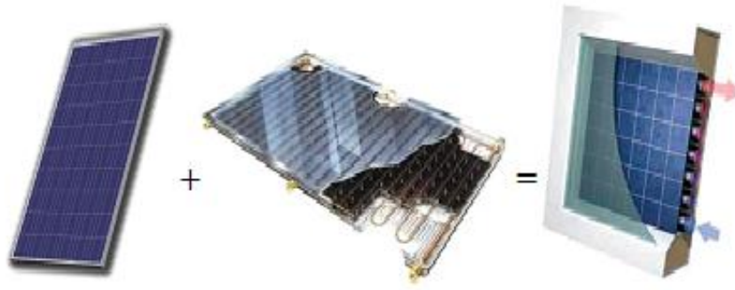
Fig. 5. Photovoltaic-thermal technology concept.
