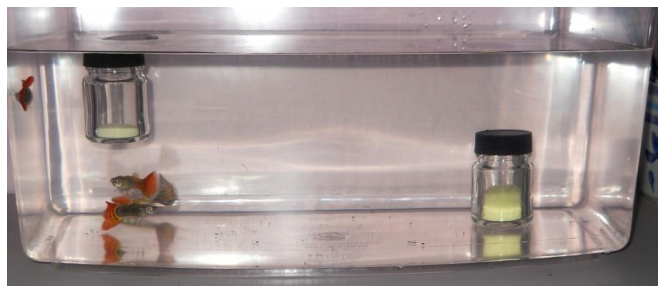
Fig. 7. Aquarium with excited (left) and nonexcited (right) phosphors.
