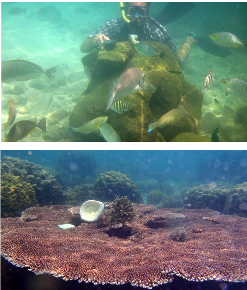
Fig. 8. Installation of a concrete matrix covered by \text{SrAl}_2\text{O}_4:\text{Eu}^{2+} , \text{Dy}^{3+} on the stone (top) and on the real corals (bottom).
